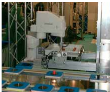
An RH-6SH in a palletising application
